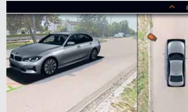
The Parking Assistant with Reversing Assistant can handle the most difficult parking spots with ease. You can go in and out of parking spots with precision while the system controls the steering, you still have control of the accelerator, gears, and brakes.
