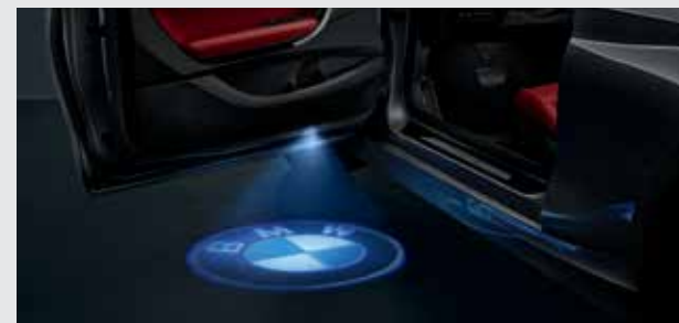
BMW LED Door Projectors. The innovative door projectors are automatically activated when the doors are opened. They project an image onto the ground next to the car using an interchangeable slide.
