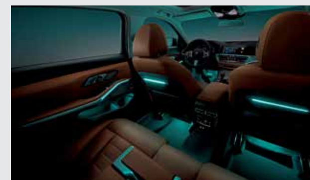
Ambient Light , including ambient contour lighting in the front and rear doors as well as in the back of the front seats, creates a relaxed, cosy lighting atmosphere in the interior. The six dimmable lighting designs also include a dynamic function in four applications. The Welcome Light Carpet illuminates the area in front of the vehicle doors when getting in and out.
