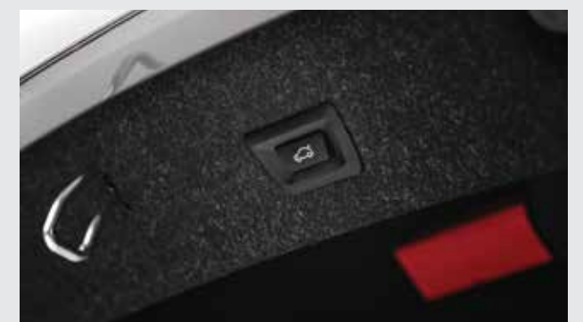
The Automatic Tailgate opens and closes at the press of a button from within the vehicle, as well as with the vehicle key. An additional button for closing the tailgate is located on its exterior.
